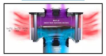
What we fools can't do, other companies, see above, can generate a supply air temperature of 17.5°C from outside air of 40°C at a wet bulb temperature of 20.8°C and that only with a heat exchanger and an Oxycom humidifier in the air conditioner, i.e. without
