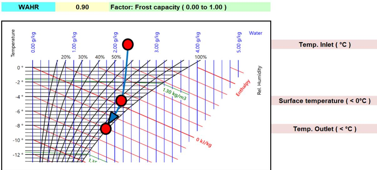
The airside reported **pressure drop depends on the degree of icing** and is controlled by the defrost interval in hours. If you change this interval, one of the two following macros must be executed. The same applies to changes in the heat exchanger parameters such as fin pitch, number of tube rows, etc.
