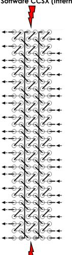
6 Tube rows on depth Piece 30 Tube rows on height Piece 18 Number of circuits(NC) Piece Tube arrangement **InLine** Left Air flow direction Order Number 180 **Tubes Total** 10 Tubes in series 0 **Tubes Blank**
